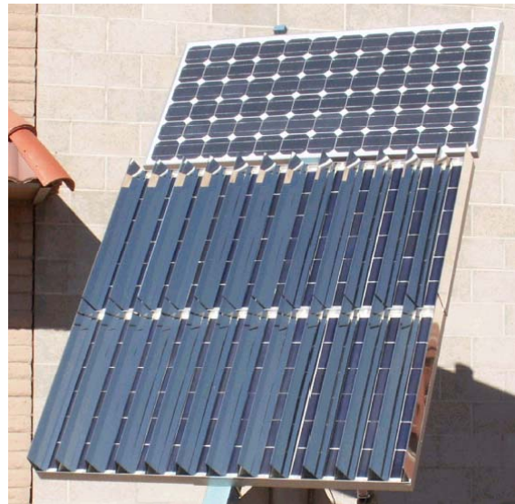
Figure 4: Two JXC 3s-180 modules and one Sharp 175 W module on 2-axis tracker in Albuquerque NM.
