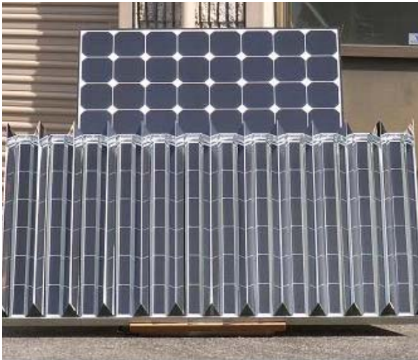
Figure 4: TOP JXC 3s-180 module design and BOTTOM Photo of first fabricated panel.
