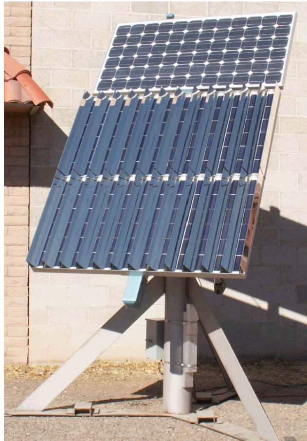
Figure 5: Two JXC 3s-180 modules and one Sharp 175 W module on 2-axis tracker in Albuquerque NM.
