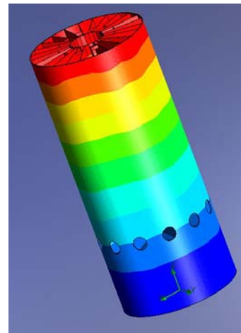
Figure 10: Temperature profile for recuperator.
